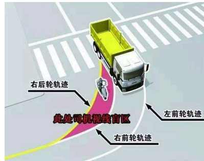
Figure 1: Right turn blind spot of truck
