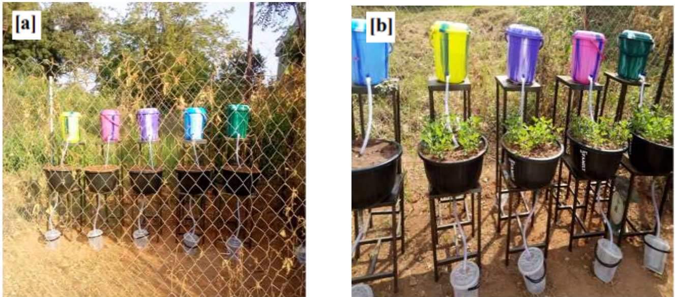
Figure 2a & 2b: A set of weighing lysimeters during experimentation and crop growth
