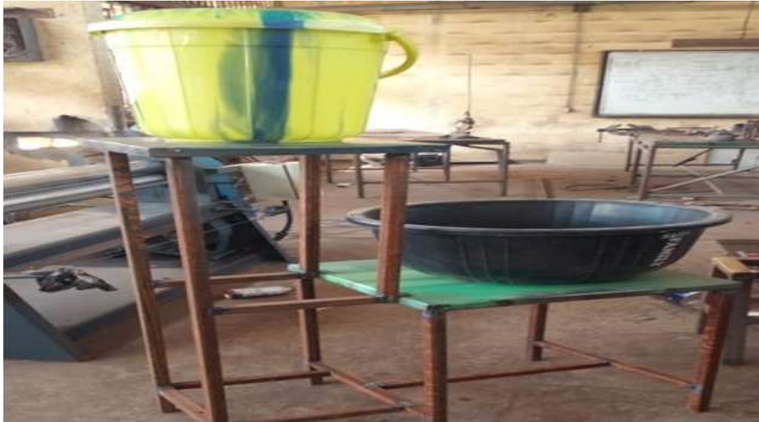
Figure 1: Weighing lysimeter during construction
