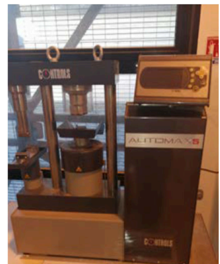
Figure 2.b: Press using for splitting tests
