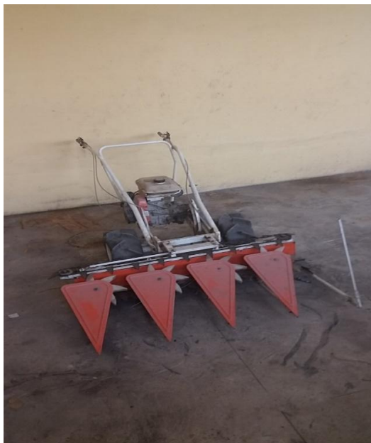
Figure 1: Walk behind motorized rice reaper
