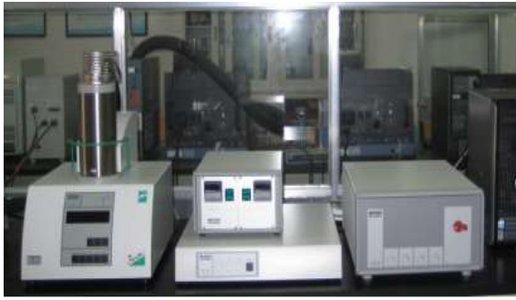
Figure 1: STA-449C synchronous thermal analyzer
