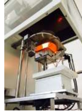
Figure 2: Cone calorimeter table
