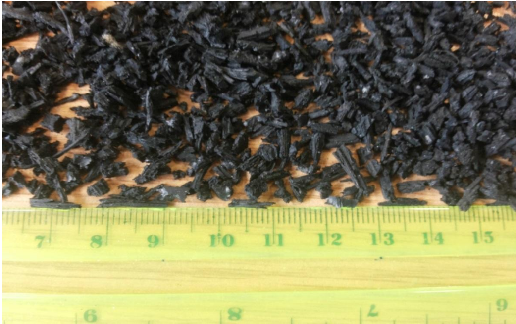
Figure 2: Crumb rubber (8mm length) particles from worn out tyres
