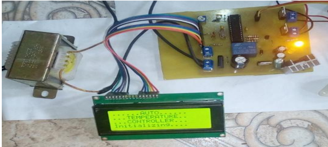
Figure 12: LCD Initialization process of the system setup
