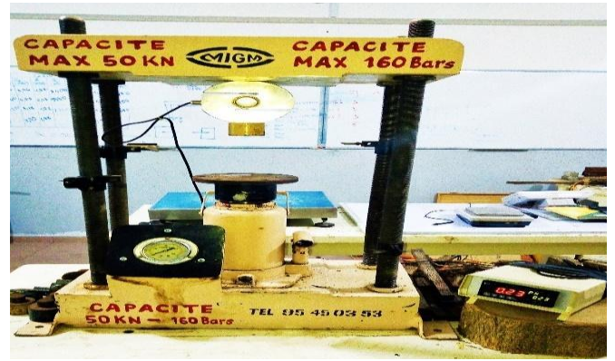
Figure 2 : Press for measuring the compressive strength
