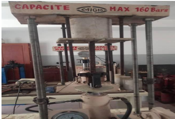
Figure 1: Pull out device (Standard SN EN 14488-4)
