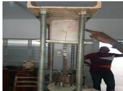
Figure 12: View showing a crack in the concrete after testing
