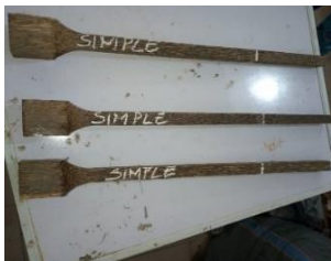
Figure 3: Single Borassus stems (control tubes)
