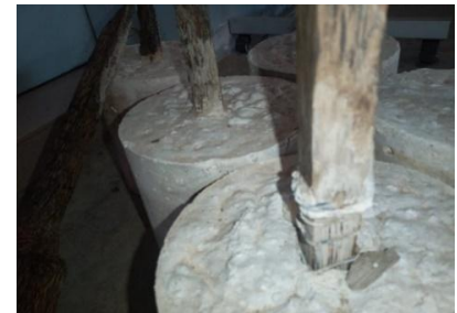
Figure 13: View showing the break between the stem and the concrete marked by the tearing of the annealed wire after pull out test
