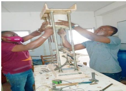
Figure 11: Laying a test specimen in the pull out machine
