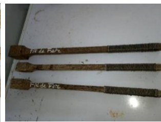
Figure 5: Borassus stems wrapped in annealed wire
