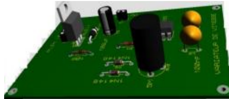
Figure 20: 3D view of the disposing of DC DC conveter's components on printed circuit card
