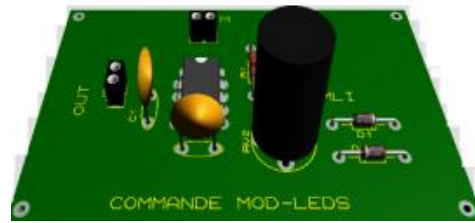
Figure 18: 3D disposition of DC DC converter's components
