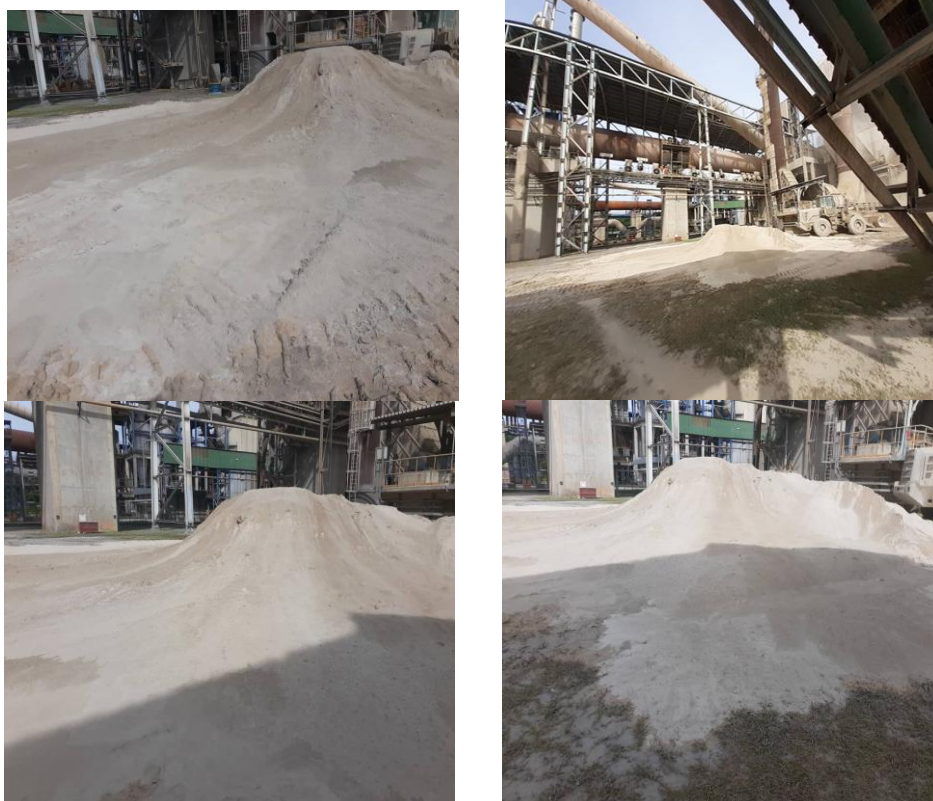
Plate No. 5: Production Plant and its Waste Cement Kiln Dust
