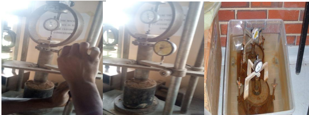
Plate No. 10: The soaked CBR Test and CRB setup in the soaking container
