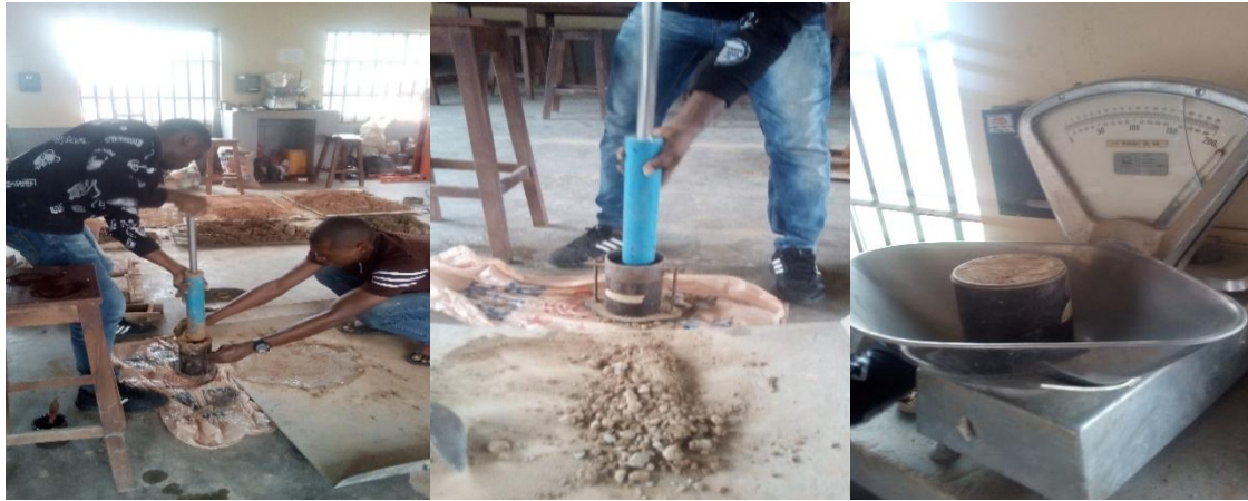
Plate No 9: Compaction test analysis
