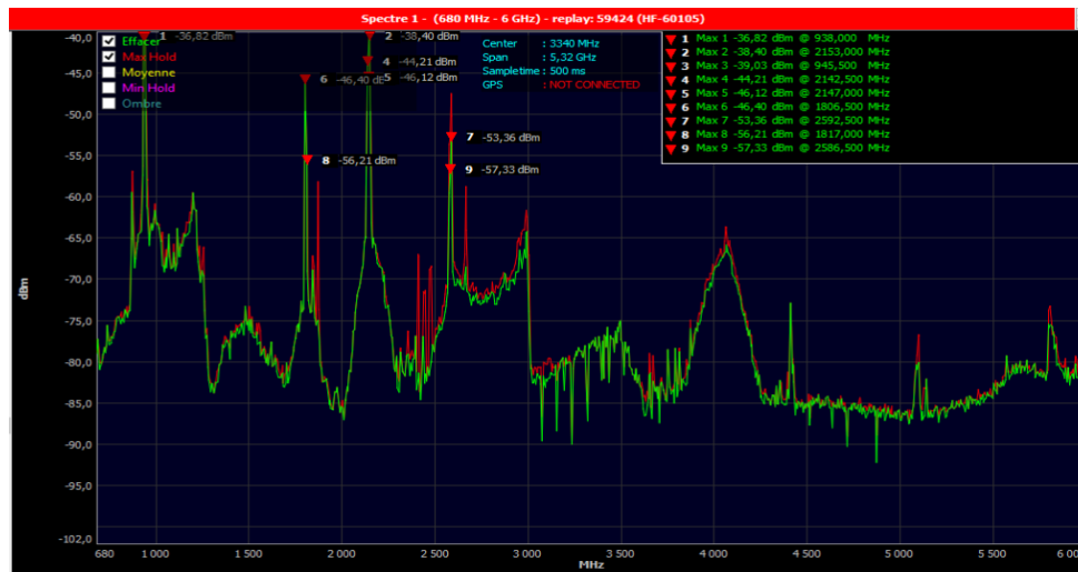
Figure 4: Total power of the electromagnetic field
