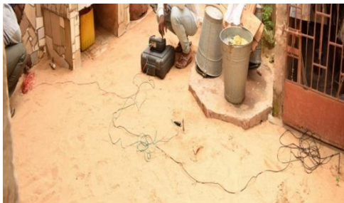
a) Arrangement of stakes and cables on the device
