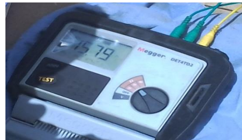
b) Earthing resistance value displayed by the device
