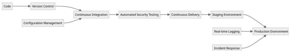
Figure 5: Low-Level Architecture Diagram of the DevSecOps Pipeline
