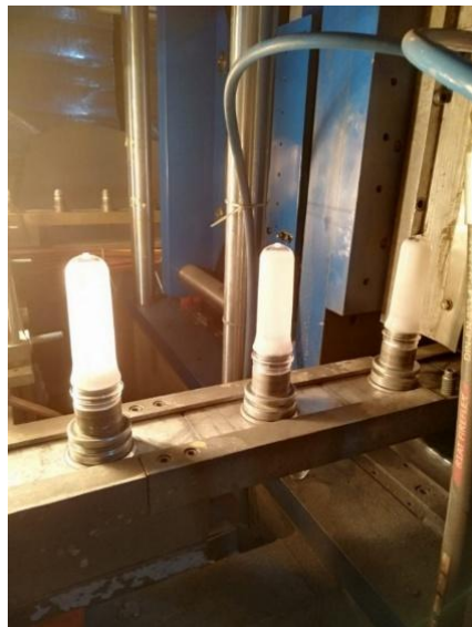
Figure 8: Burnt and wasted preforms
