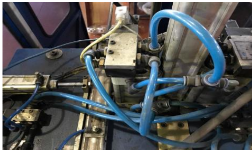
Figure 3: Initial mechanism of the top plate of the clamp driven by pistons
