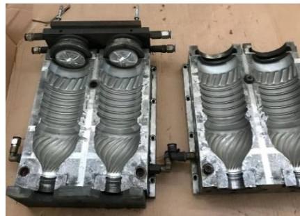
Figure 2: A sample of multi cavity mold type used in the experiments
