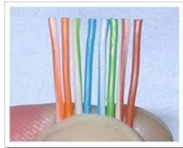
Figure 6: Arranging the Category 5 Cable According to 568B Standard
