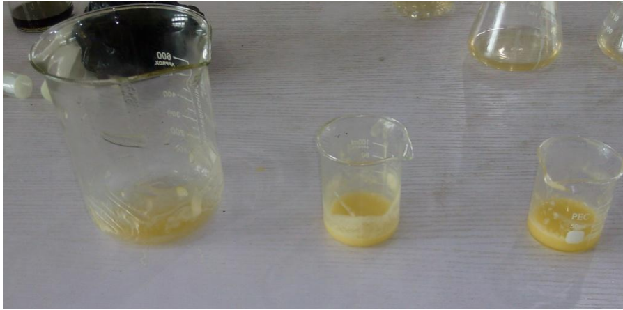
Figure 7: Formation of emulsion with sodium silicate samples
