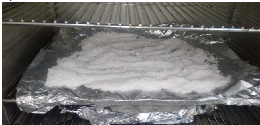
Figure 9: The produced detergent dried in oven
