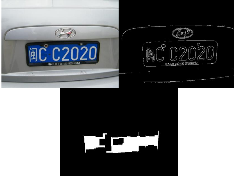
Figure 2: Original image, edge detection effect, dilation effect
