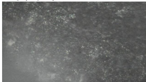
Figure 6: The Micrograph of Agbaja Iron reduced @ 1000 °C (Fully reduced)
