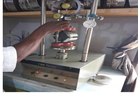
Plate 2.4: placement of specimen in breaking head (CBR tester machine)
