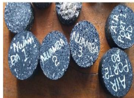
Plate 2.12: After compaction of cored samples
