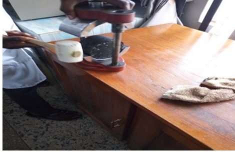
Plate 2.3: placement of specimen in mold
