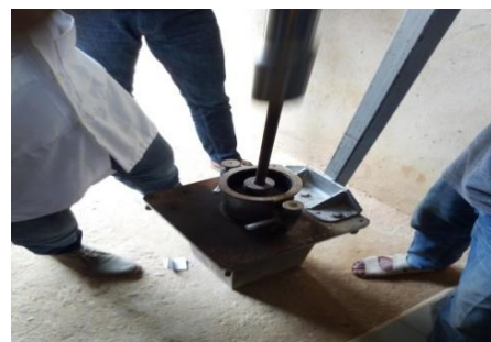
Plate 2.2: Compacted fresh asphalt specimen
