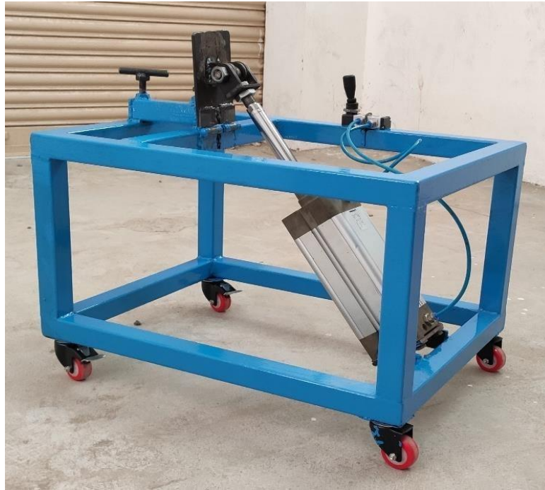
Figure 10: Working diagram of a pneumatic bending machine
