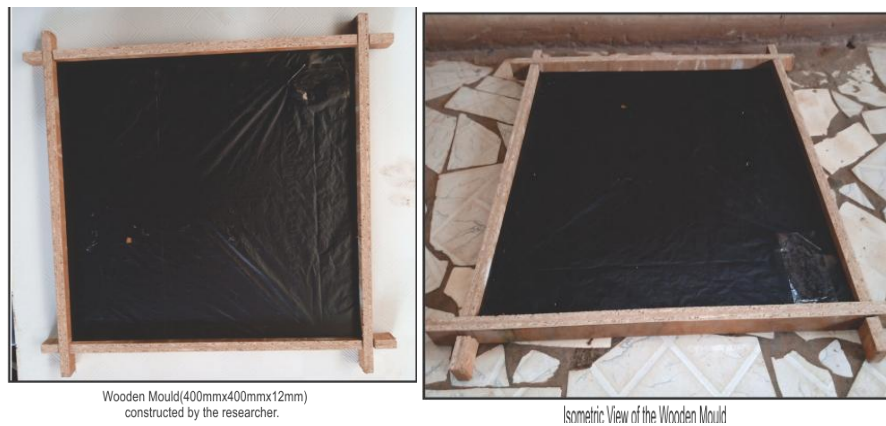
Figure 1: 400x400 by 12mm Wooden Mould
