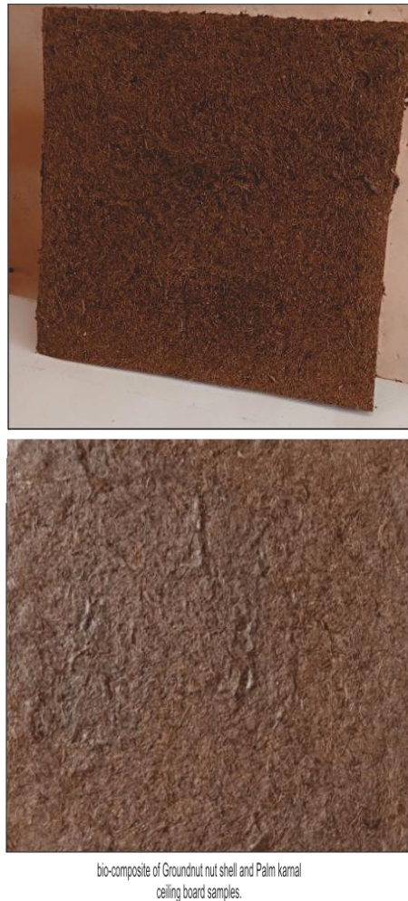
Figure: 2. Bio- composite of Groundnut Shell & Palm kernel Ceiling Board
