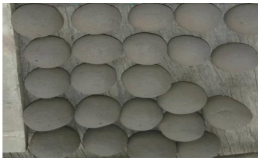
Figure 2.7 : Some produced pellets from Itakpe Iron Ore
