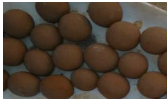
Figure 2.8: Some produced pellets from Agbaja Iron ore
