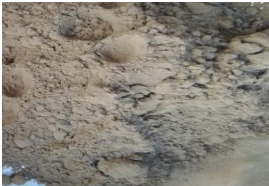
Figure 2.5: The pulverized Itakpe iron ore
