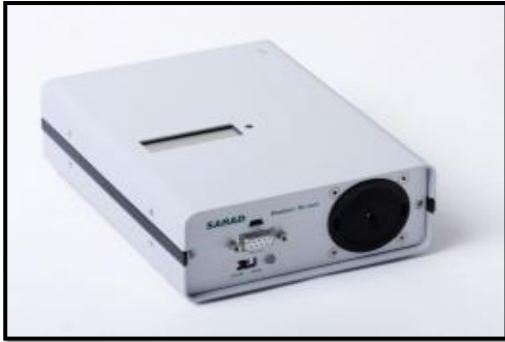
Figure 2: A portable device Radon Scout Plus meters
