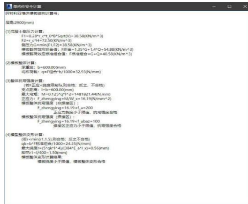
Figure 3: Output interface of safety calculation book of wall frame panel
