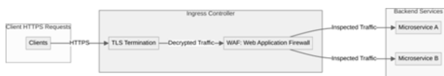
Figure 1. Proposed Architecture for Securing Ingress Traffic with TLS Termination and WAF Integration.
