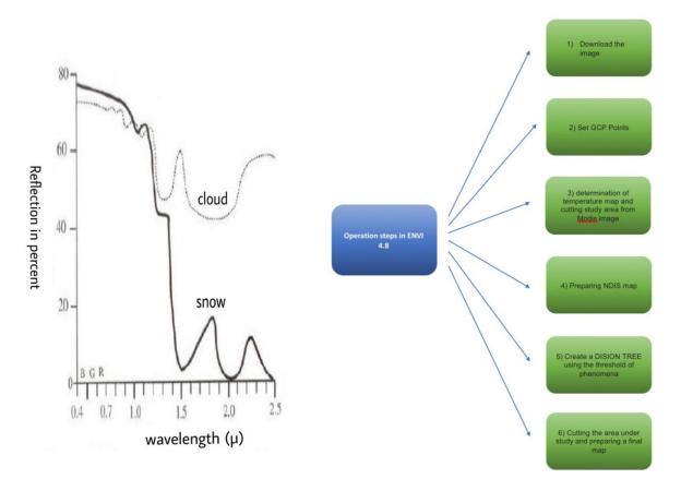
Figure 2: Spectral Reflection Curve of Snow and Cloud
