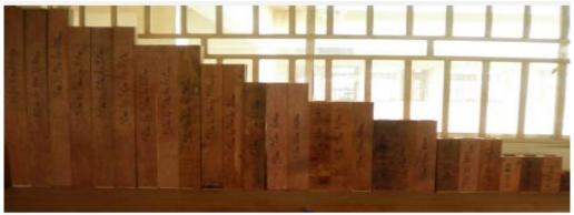
Figure 2.2: Photograph of formworks showing dimensions 50 x 50 x 50) mm and above
