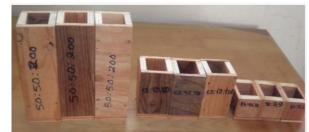
Figure 2.1: Photograph of formworks showing dimensions 50 x 50 x 200 mm and below
