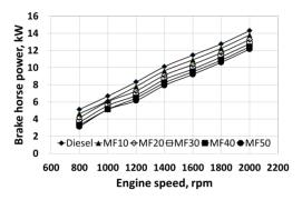
Figure 2: Brake horse power versus engine speed for various fuels
