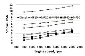
Figure 6: Smoke versus engine speed for various fuels
