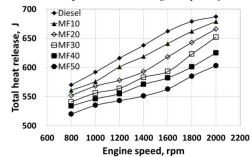
Figure 3: Total heat release versus engine speed for various fuels
