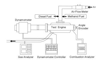
Figure 1: Schematic diagram of experimental apparatus
