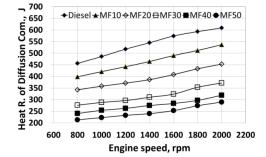
Figure 4: Heat release of diffusion combustion versus engine speed for various fuels
