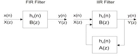
Figure 1: Block diagrams of FIR and IIR filters
