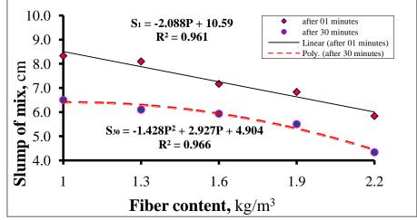
Figure 2: Relationship between fiber content and slump
