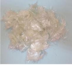
Figure 1: Polypropylene fiber
