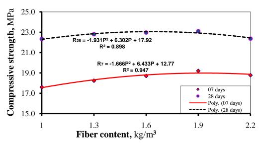
Figure 3: Relationships between fiber content and compressive strength
