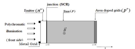
Figure 1: Silicon Solar Cell structure to the  $n^+pp^+P$  type under magnetic field and polychromatic illumination
