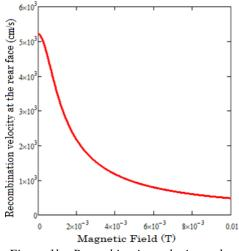
Figure 1b : Recombination velocity at the rear face Sb<sup>\*</sup> versus magnetic field
