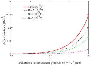
Figure 5: Series resistance versus junction recombination velocity for different values of the magnetic field.  $D=26cm^2/s, \ \mu=10^3cm^2.V^1s^{-1}, \ \tau=10^{-5}s, \ H=0,03cm)$
