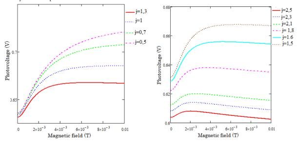
Figure 2: Photovoltage versus magnetic field for different values of the junction recombination velocity near the open circuit
