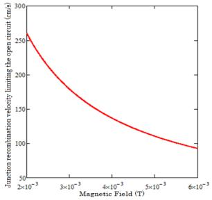
Figure 4: The junction surface recombination velocity of minority charge carriers limiting the open circuit versus of magnetic field  $D=26cm^2/s, \mu=10^3 cm^2 V^1 s^{-1}, \tau=10^{-5}s, H=0,03cm)$
