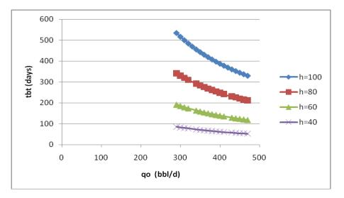
Figure 4: Effect of Production Rate on Breakthrough Time at varying Reservoir Thicknesses
