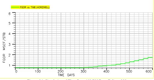
Figure 14: Simulation of Flow Rate 460 Bbl/D on Eclipse 100
