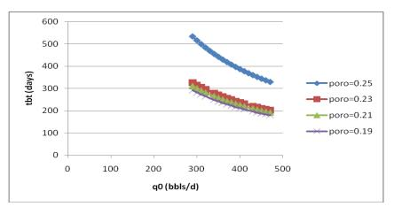
Figure 5: Effect of Production Rate of Breakthrough Time at varying Reservoir Porosities
