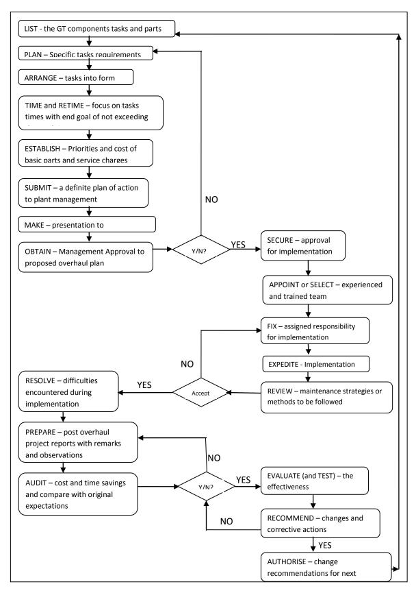
Figure 1 Gas Turbine Overhaul Value Analysis Flow Diagram
