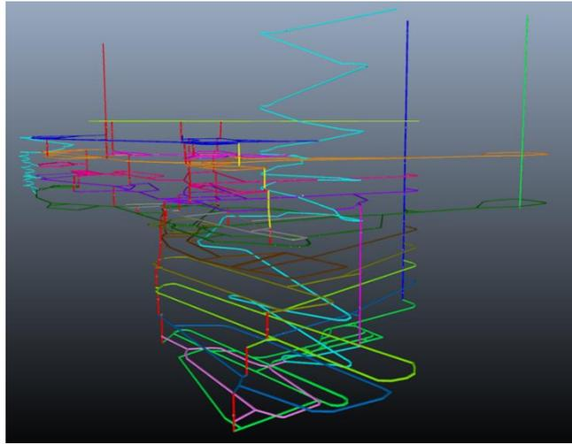
Figure 1: Three-dimensional ventilation network model of Anqing Copper Mine
