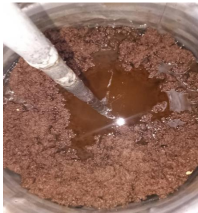
Figure 12: Kneading process completed ready to separate oil
