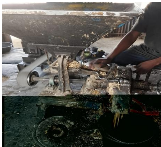
Figure 10: Grinding Process of the Groundnut Seed into Groundnut Paste
