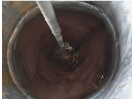
Figure 11: Kneading process, system loaded with 20 Kg ground nut paste
