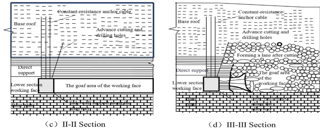
Figure 2: Process Flow Chart of the Methodology for Cutting Top and Implementing Pressure Relief while Leaving Intervening Roadways along the Mining Face
