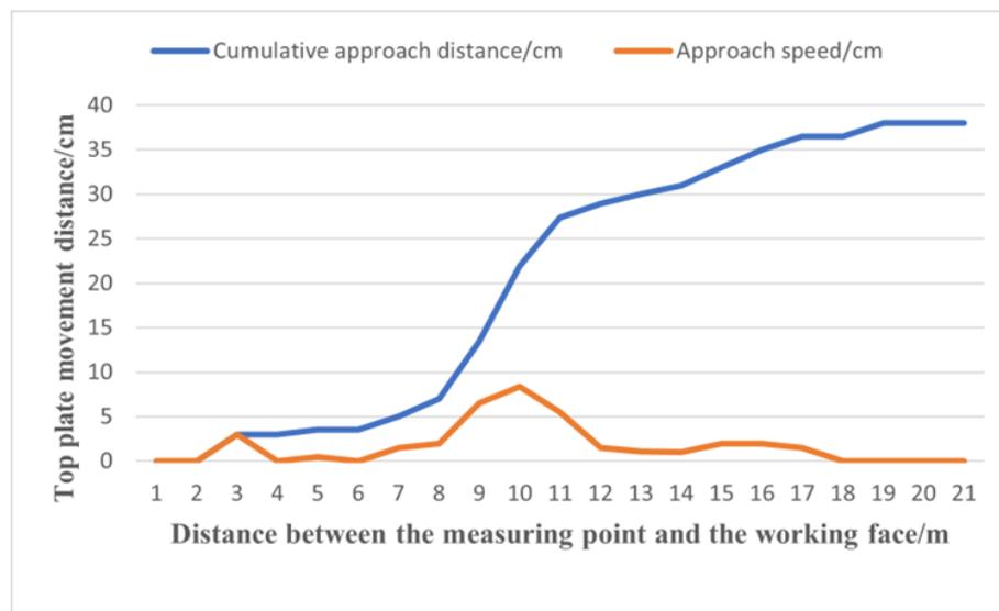
Figure 4: Diagram of the trend of roof displacement variation
