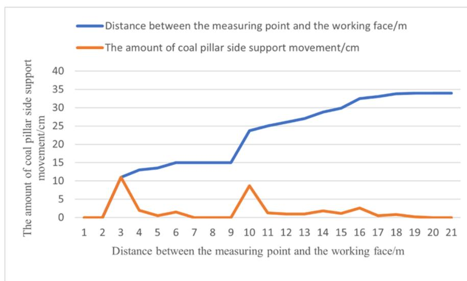
Figure 6: Trend Chart of the Variation of the Distance of the Roof Support Movement in the Coal Pillar Area
