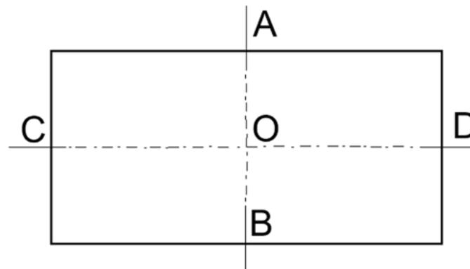
Figure 3: Layout of Measuring Points for Monitoring the Displacement of Surrounding Rock in the Retaining Shaft
