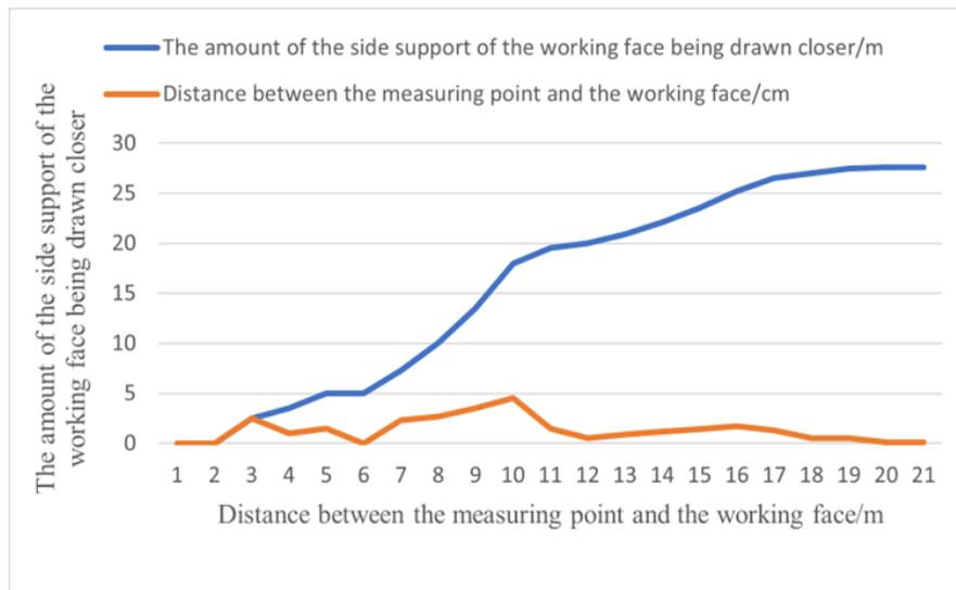
Figure 5: Trend Chart of the Distance of the Side Wall of the Working Face Moving Closer
