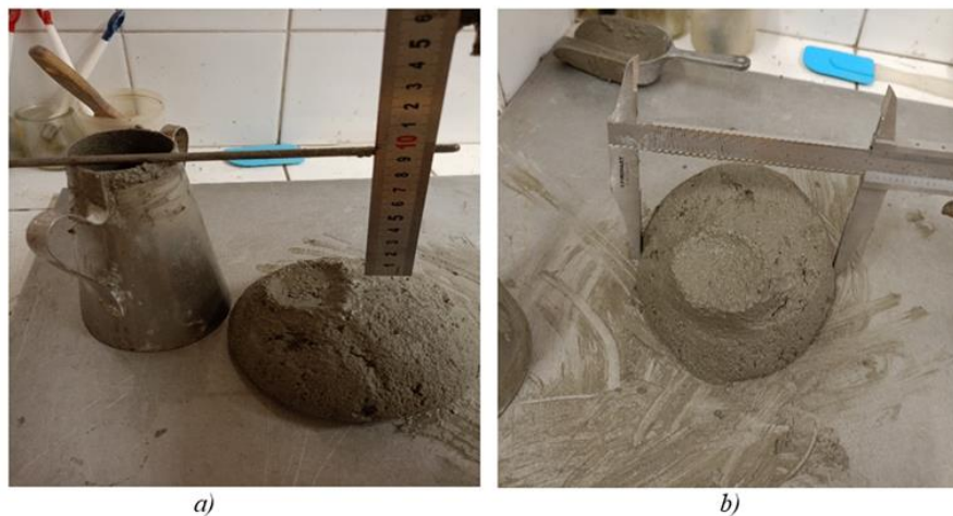
Figure 9: a) Mini-cone slump measurement, b) Mini-cone spread measurement
