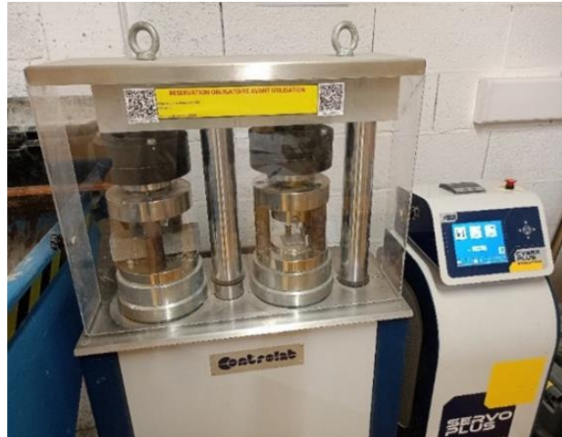
Figure 10: Controlab press for flexion-compression at INSA Rennes
