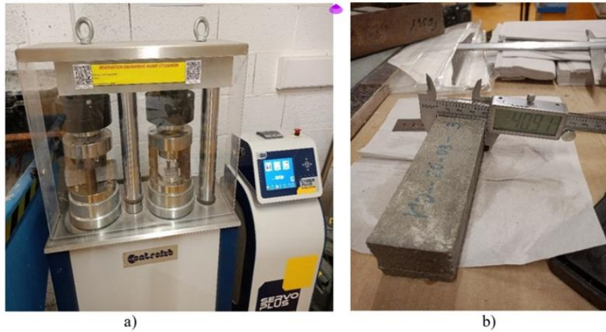
Figure 14: a) Controlab press for flexural-compressive strength tests and b) Specimen size measurements with calipers
