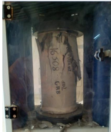
Figure 2-b: Crushing of concrete specimens
