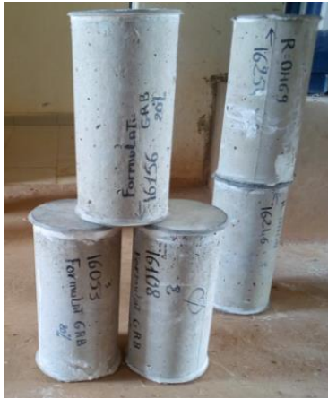
Figure 2-a: Ready-mix concrete specimens
