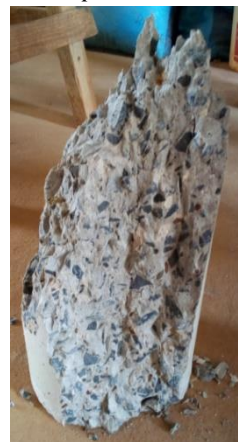
Figure 2-c: Interior appearance of crushed specimens
