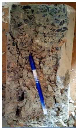
Figure 2-c: Interior appearance of crushed specimens
