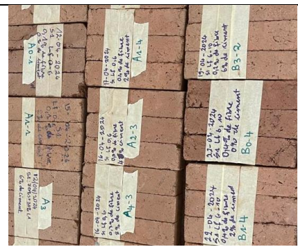
Figure 4: Test specimens 4x4x16 cm 3
