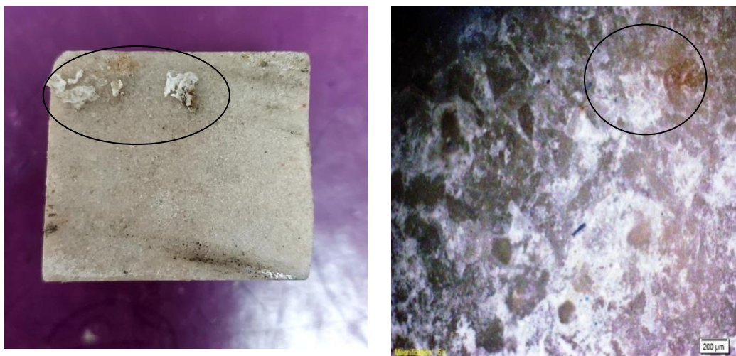
Figure 12: Surficial efflorescence associated with salt crystallization test of the studied sample and illustrated by elliptical shape (left). Stereo-photomicrograph shows slight Surficial efflorescence crystals associated with salt crystallization and marked by circle (right).
