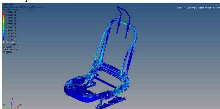
Figure 11: Stress nephogram under equivalent 530Nm load after lightweight
