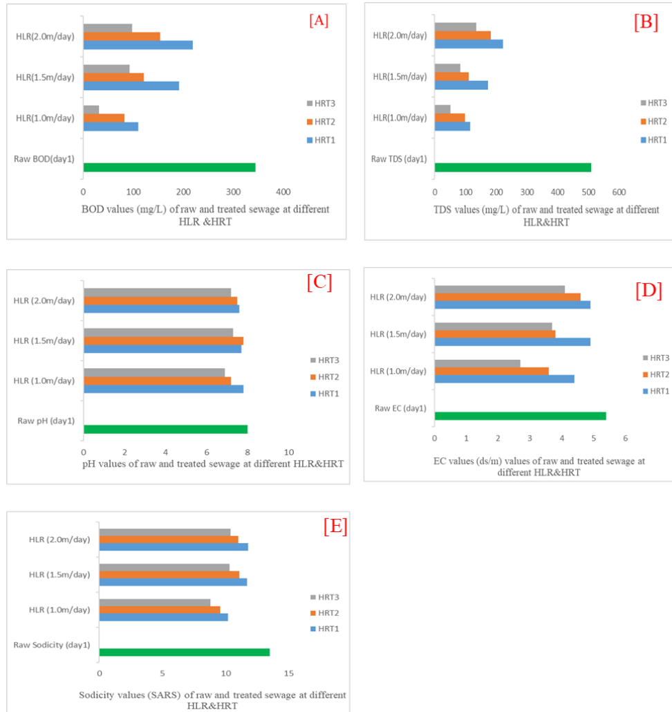
(A) BOD values of raw and treated sewage water (B) TDS values of raw and treated sewage water (C) pH values of raw and treated sewage water (D) EC values of raw and treated sewage water (E) Sodicity values of raw and treated sewage water.
