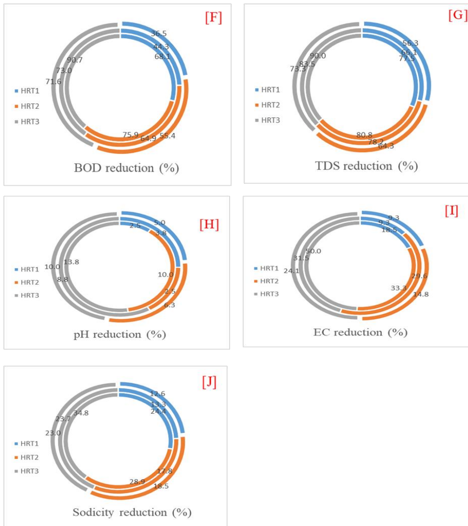
F, G, H, I & J): Impacts of HLR & HRT on BOD, TDS, pH, Electrical Conductivity and Sodicity reduction of the treated sewage water.
