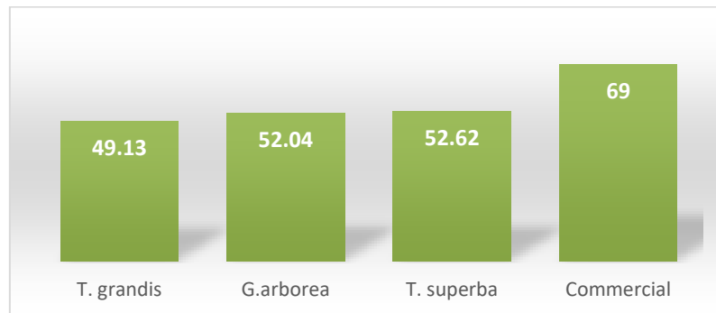
Figure 4.6: Comparison of Ash Content of Sawdust-Reinforced Composite and Commercial Brake Pads.
