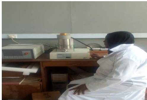
Plate 3.1: Differential Thermal Analysis (DTA) Setup for the Thermal Properties of the Brake Pads
