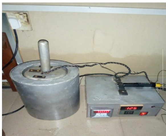
Plate 3.2: Determination of Thermal Conductivity of the Brake Pad Sample
