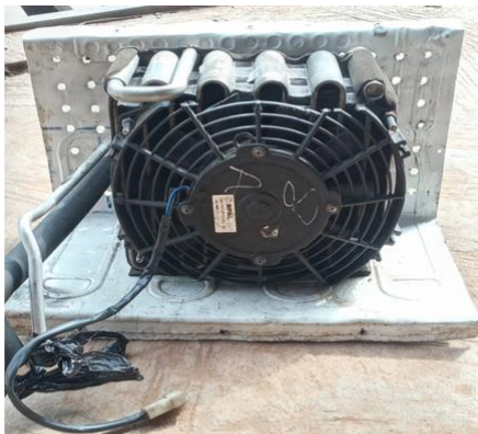
Plate 6: Assembly of the evaporator and blower motor(fan)
