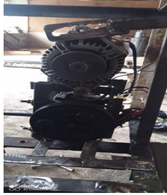
Plate 3: Installation of the Compressor and the Alternator
