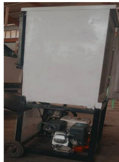
Plate 7: Assembled Vaccine Refrigerating system.
