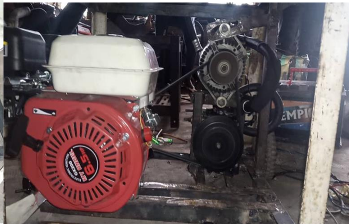
Plate 2: Aligning the alternator compressor and the Engine
