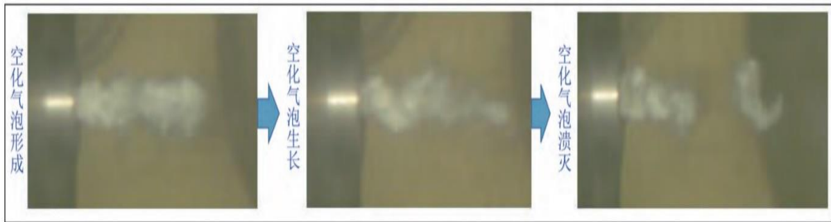
Figure 4: Mechanism of cavitation effect of ultra-high pressure water jet
