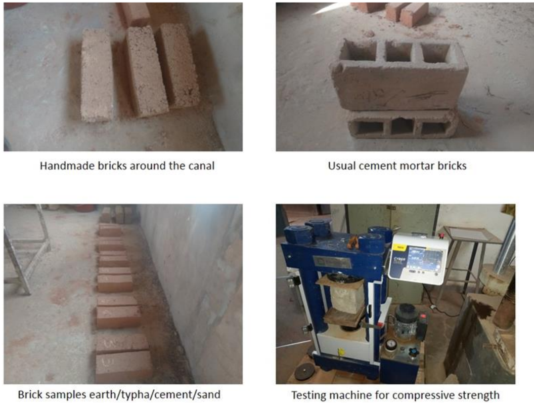
Figure 4: Samples, comparison bricks and test machine
