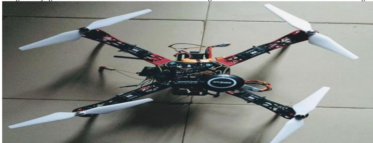
Figure 8: Propellers installation Source: [2;4;6]
