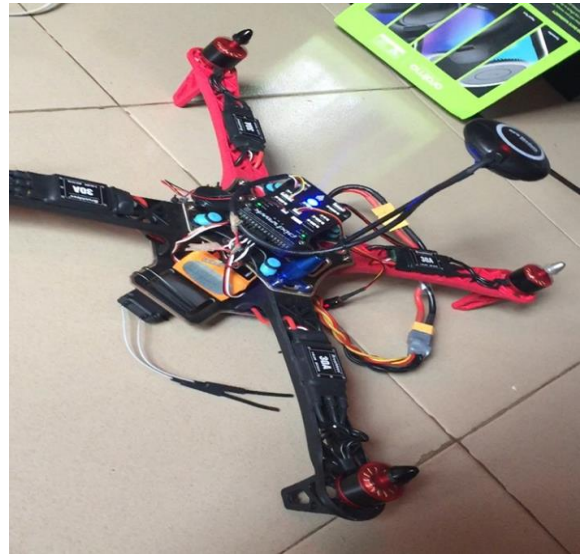
Figure 7: Pixhawk installation and GPS mounting
