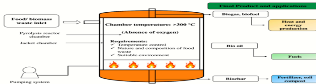
Fig. 5. Mechanism of pyrolysis process with their final products and applications.
