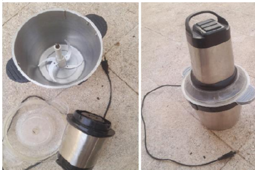
Figure 2: Multifunctional grinder. A. grinder different parts. B. grinder assembled
