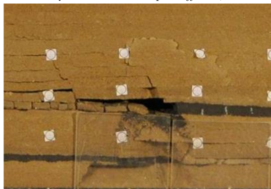
( c ) The working face is located directly below the boundary of the goaf ( local amplification map )
