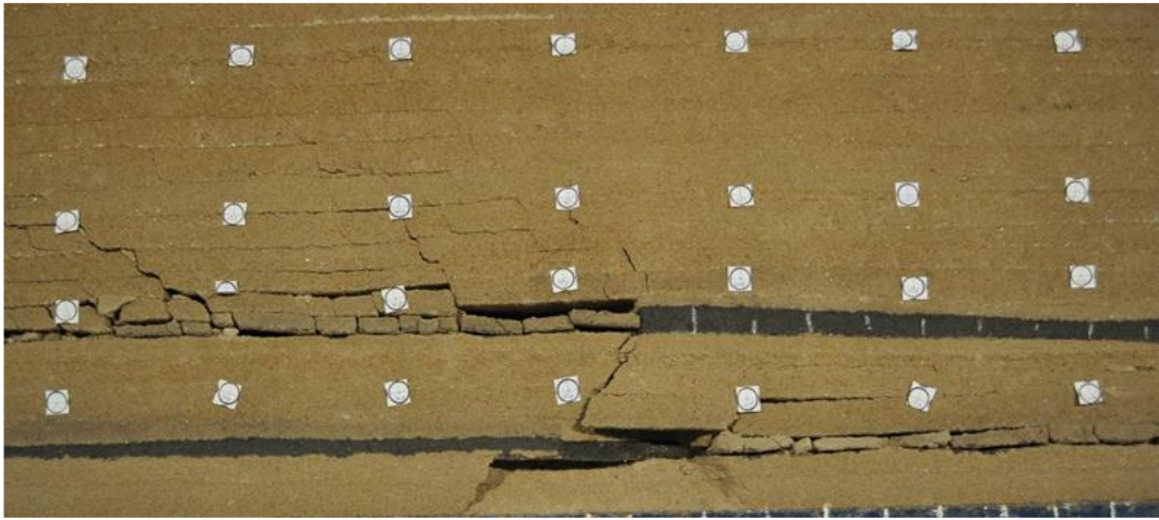
( b ) Working face is ready to enter 31201 open-off cut ( local enlargement map )
